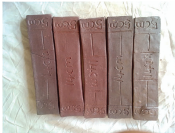
Fig. 6. The shrinkage test.
