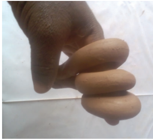
Fig. 5. The plasticity test.
